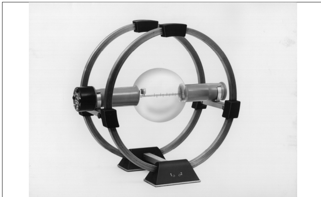
Fig. 1: 06959-00 Narrow-beam tube 06959-00 in pair of Helmholtz coils 06960-00
